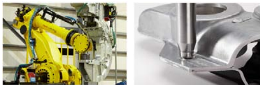
Fig. 1. Friction Stir Welding System of Honda (Japan)
