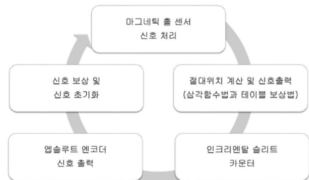
Fig. 1. Flow chart for magneto-optical encoder
