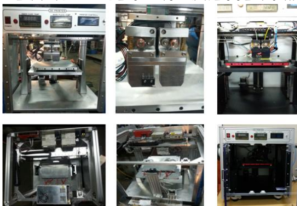
Fig. 1. Dual nozzle set for extruding model and soluble support material
