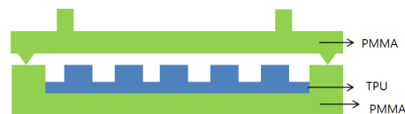
Fig. 1. A schematic of micro fluidic device
