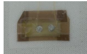
Fig. 3. Photograph of GSR sensor composed of core-shell nanowires
