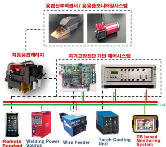
Fig. 1 Schematic diagram of integrated auto-welding system
