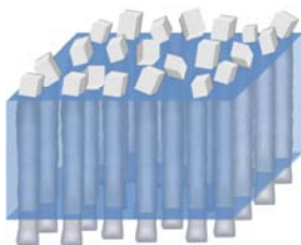
Fig. 2. Schematic diagram of GSR sensor based on Ag-AgCl core-shell nanowires
