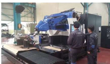
Fig. 2. Developed FSW machine with parallel kinematic structure
