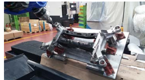
Fig. 3. Friction stir welding of Al-Steel rear cross member
