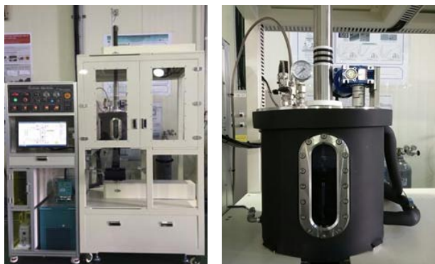
Fig. 1. Desalination test unit and dual cylinder type hydrate reactor
