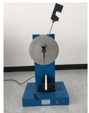
Fig. 2 3-point bending test apparatus Fig. 3 Charpy impact test apparatus
