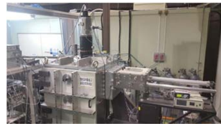
Fig. 1 Photograph of low vacuum high voltage e-beam equipment for metal heat treatment
