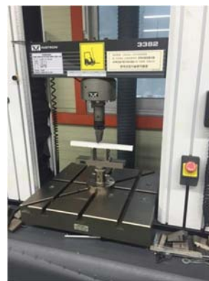
Fig. 2 3-point bending test apparatus Fig. 3 Charpy impact test apparatus
