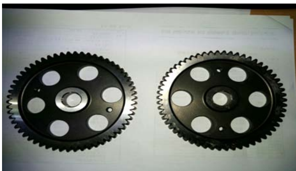
Fig. 1. A normal Gear Psalms (left) defective Psalms (right)
