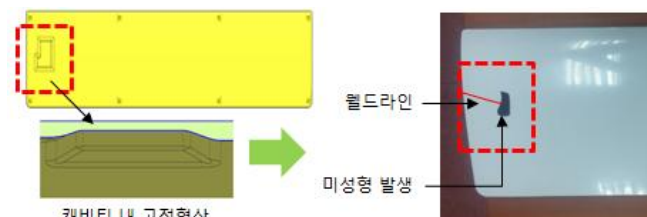
Fig. 2. Defect in the case of fixed core
