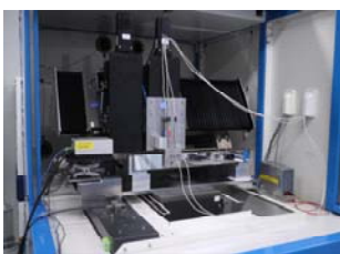
Fig. 1. Measurement set up for motion errors of hybrid machine
