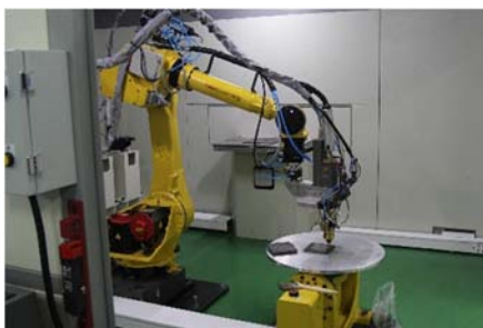
Fig. 1 Laser cladding system using multi-axis robot
