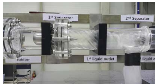
Fig. 4. Experimental result; swirl flow inside separator.
