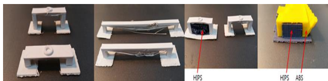
Fig. 2. Overhanging structure supported by soluble HIPS structure
