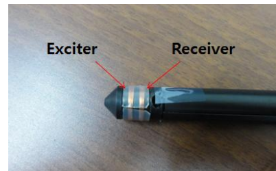
Fig. 2 ECT sensor manufacture for detecting inner cracks
